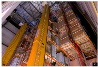
New robotic technologies implemented in warehouses make it possible to densify goods by using the entire height of the buildings.
