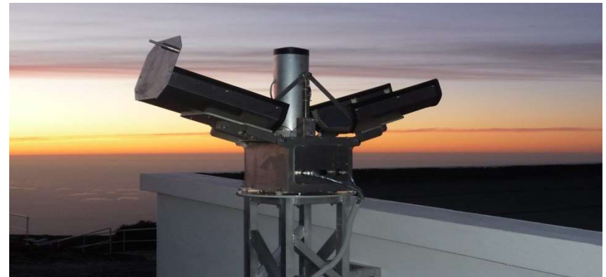
AMOS created by astronomers from the CU monitors southern sky and determines the trajectories of meteors
