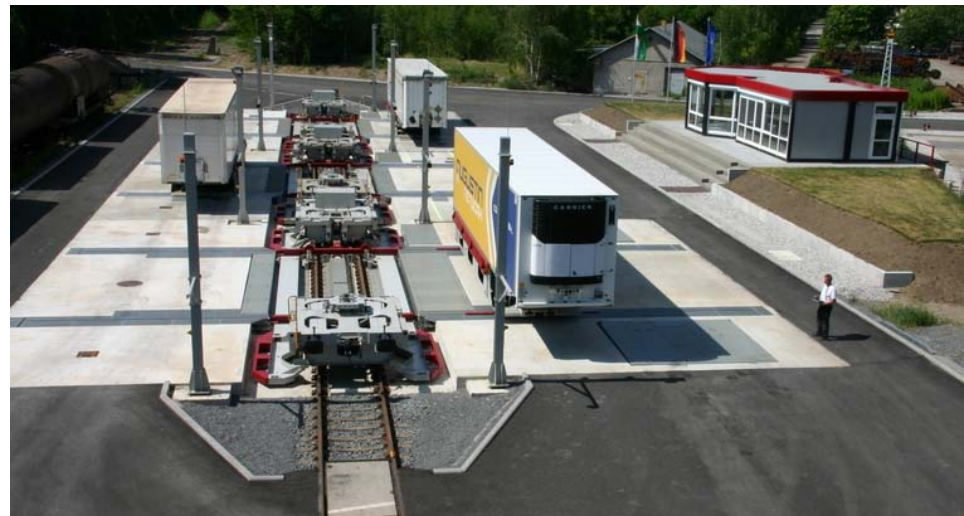
Automated and parallel transshipment process (CargoBeamer, DE)
