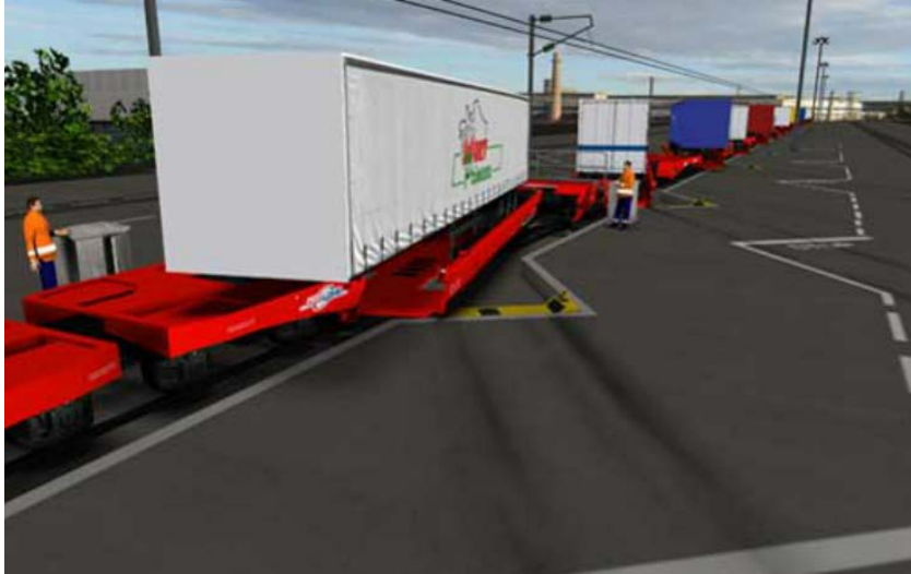
Low-floor articulated railway Wagon (Modalohr, FR)
