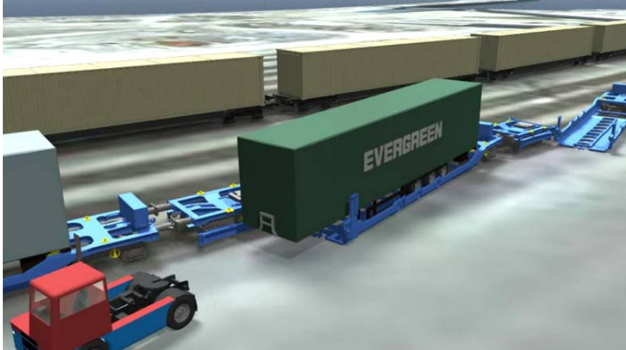
Freight wagon with a swingable pocket (Kockums Industrier, SE)
