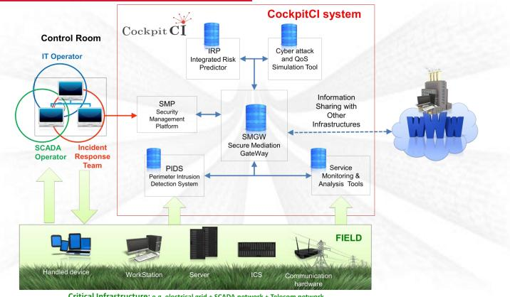
Critical Infrastructure: e.g. electrical grid + SCADA network + Telecom network
