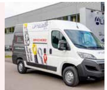
appointment has been fixed, the LIFTEUROP technical representative comes on site. The accessories are checked on a test bench installed in a dedicated vehicle, where it can be repaired and put back into service immediately.
