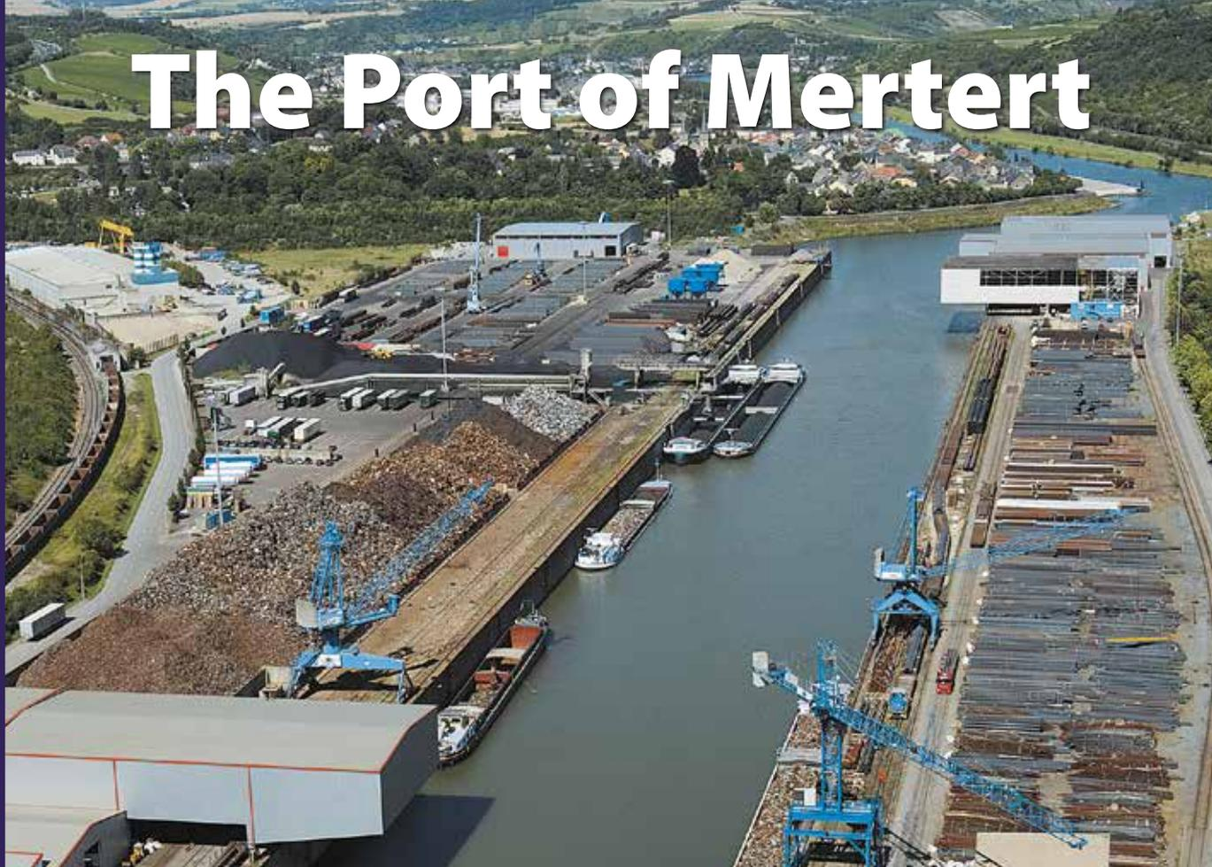
Located on the municipalities of Mertert and Grevenmacher on the left bank of the Moselle, the Port of Mertert has a total area of 65 hectares. Both docks along the port basin, on which are installed 11 rolling cranes with a lifting force of 12 to 124 tons, have a total length of 1,600 meters. The transshipped products are mainly steel products upon arrival and departure of Arcelor-Mittal plants installed in Luxembourg, petroleum products, agricultural products and construction materials.
